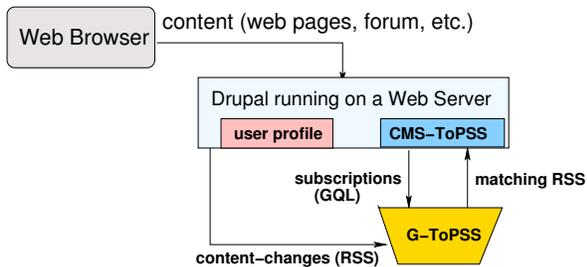
Figure 7: CMS-ToPSS system architecture
